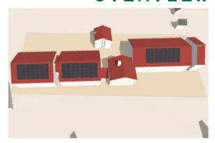
Abigail Court Care Home, operated by Luton Borough Council, has invested in a solar PV and battery storage system to cut operating costs and improve its environmental performance. The 46.575 kWp installation combines 115x Viridian high efficiency solar panels with integrated battery storage, providing the facility with clean renewable energy, reduced grid reliance, and long-term financial savings.
