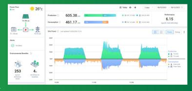
standards of compliance and quality. Once operational, the system was integrated with SolarEdge's advanced monitoring platform, giving the Academy real-time insights into energy generation, onsite consumption, and exports to the grid.
